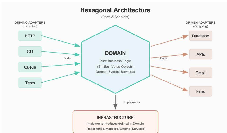
*Hexagonal Architecture diagram showing the domain at the center of a hexagon, with incoming adapters (HTTP, CLI, Queue, Tests) on the left side and outgoing adapters (Database, External APIs, File System) on the bottom*
